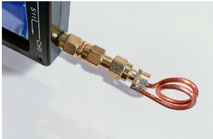
Construct small loop attached to SMA connector
